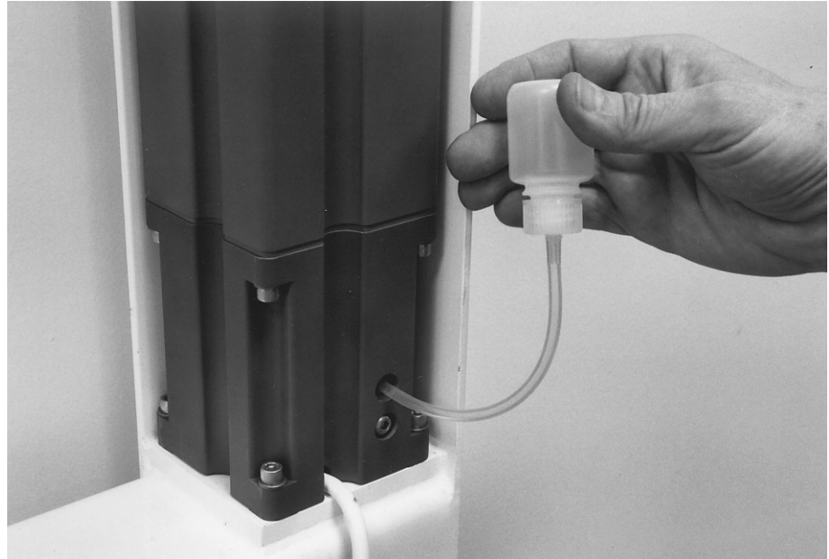
Figure 2.3 — Horizontal Damping Oil Installation
