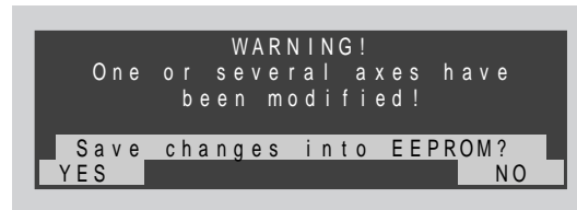
Fig. 1.15 — Save screen for axis modifications.
