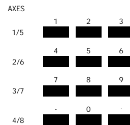
Fig. 2.3 — The rows of the numeric keypad indicate the axis that will JOG.
