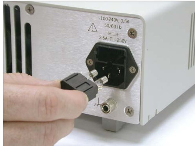
Figure 10: Removal of Fuse Block.
