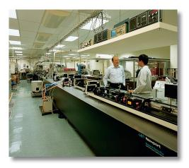
Figure 1: Newport table systems minimize the relative motion of a large array of sensitive scientific and production equipment
