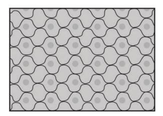
Figure 3: Ordinary small-cell core
