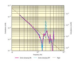
**Figure 7:** Dynamic compliances near the corner of the table. Red line: damping on; Blue line: damping off, dots: rigid body line. Table size: 8 ft x 4 ft x 12 in.
