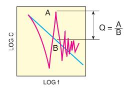
Figure 6. Maximum amplification at resonance (Q).
