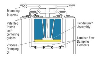
Figure 25: Diagram of Newport's patented horizontal isolation piston.
