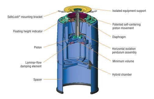
Figure 16: Section view of a Stabilizer S-2000 Isolator.
