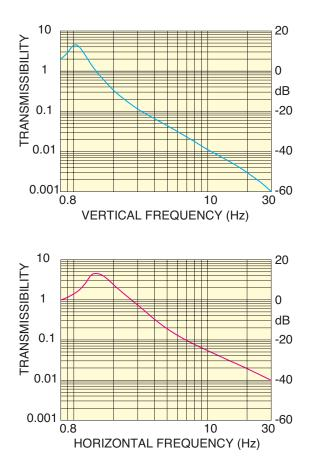
For example, given a system with a 2 Hz natural frequency; and thus a transmissibility of one at 2.8 Hz  $(1.41 \times 2)$ ; the transmissibility at 28 Hz would be -40 dB, or 0.01. Horizontal isolation in a Newport isolator is achieved by use of a pendulum system. The behavior of the pendulum horizontal isolator is basically the same as that of the vertical pneumatic isolator. In this case, the pendulum natural frequency is given by:
