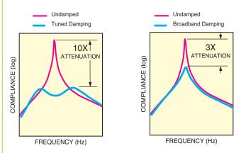
**Figure 1:** Newport tuned dampers (left) concentrate damping where it's needed most, at the frequencies of dominant resonance modes. Since broad-band dampers (right) are designed to provide moderate damping over a wide range of frequencies, they are not as effective at damping the dominant modes of table vibration.
