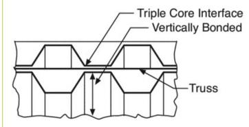
Figure 5: Trussed core design offers superior rigidity
