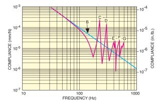
Figure 4. Compliance curve for an aluminum honeycomb core table top.
