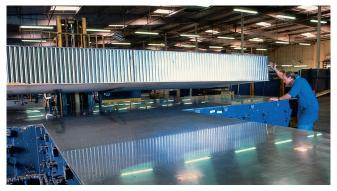
Figure 6: These precision platens allow the manufacture of large tables on a single, ultra-flat surface instead of multiple granite platens, which can compromise end-to-end flatness.
