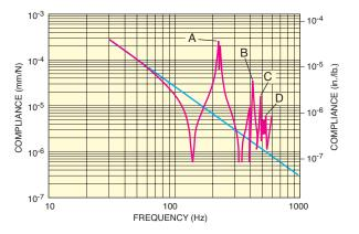
Figure 2. Typical compliance curve of an undamped table top.
