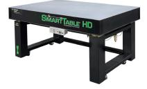
precision optical alignment and testing. The integrated accessories and ergonomic designs available with the SmartTable OTS deliver exceptional performance, flexibility and upgradability. This is the only optical table system that is field-upgradable with three levels of table damping performance and two levels of isolation performance, which could satisfy current requirements but also allow the flexibility needed for future performance improvement.
