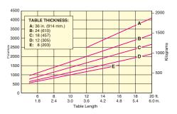
Approximate net weights ( $\pm 10\%$ ) for 4 ft (1.2 m) wide steel tables. For 5 ft (1.5 m) wide models add 20%, for 3 ft (0.9 m) models, subtract 25%. Shipping weights can be estimated by adding 100-200 lbs (45-90 kg) for crate weight.
