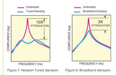
Newport tuned dampers (Figure 7) concentrate damping at the frequencies of resonance modes, where it is needed most. Since broadband dampers (Figure
