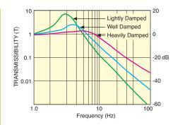
Figure 17: Transmissibility plot shows damping effects.
