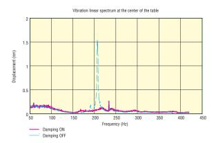
**Figure 6:** Linear spectra of vibration near the corner of the table Red line: damping on; Blue line: damping off. Table size: 8 ft x 4 ft x 12 in.
