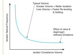
Figure 21: Isolator natural frequency vs. compliance chamber volume.
