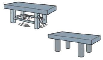
Figure 27: The tie-bars on ordinary tables can actually amplify floor vibrations.
