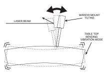
Newport's Maximum Relative Motion formula provides an excellent approximation of maximum (worst-case) table top deflection. This technical note explains and quantifies the relationship between Maximum Relative Motion and actual beam deflection in real-world applications.
