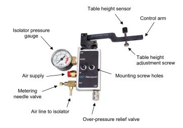
Figure 24: Newport valves are designed specifically for optical table systems.
