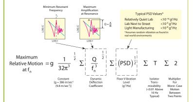
Figure 1. Formula for determining the maximum relative motion between two points on an isolated table top from any compliance curve. Table tops supported by rigid stands (or legs) would have a larger relative motion value.
