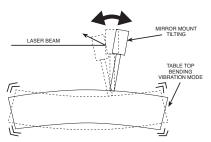
Figure 2: Table top bending is the most significant cause of beam deflection.
