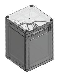
**Figure 2:** Schematic of Newport vibration absorber used in tuned damping table systems US patents 8,857,585 et al.modes of table vibration.
