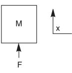
Figure 1. The free ideal rigid body model, Mx"=F
