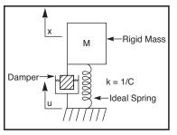
Figure 3. Damped Simple Harmonic Oscillator
