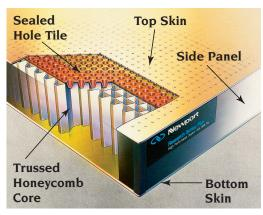
Figure 2: Honeycomb core construction creates exceptionally rigid platform for precision optical experiments
