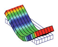
The example above shows the basic process used for determining the proper damper and location to eliminate the fundamental mode. Once the dampers are built into the table to attenuate this mode, the table is transformed from an RPR to an RS2000 with two dampers, or to RS4000 with six dampers.
