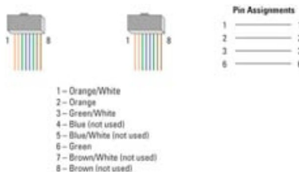
Figure 12: Straight through cables.
