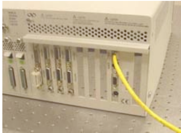
Figure 14: Direct Connection to the XPS using cross-over cable.
