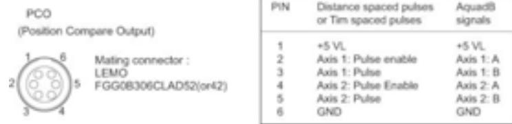
Figure 70: Position Compare Output Connector.
