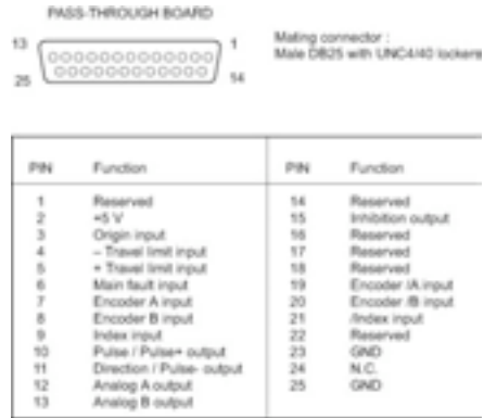
Figure 75: DRV00 Pass-Through Connector.
