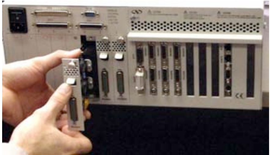
Figure 11: Installing Driver cards.
